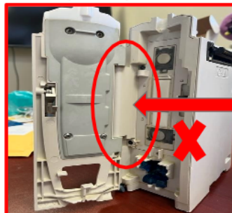
Pump Missing the Platen
